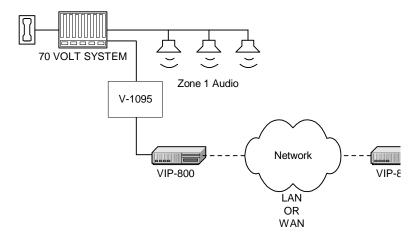
**Note:** During initial SETUP, the "Sub-Net Address" and the "Gateway MAC Number (address) of the Sub-Net Power" must be programmed in the software of each unit <u>locally</u> - on the SubNet on which the unit resides.
